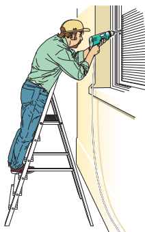
Figure 2b Correct - steps facing work activity
